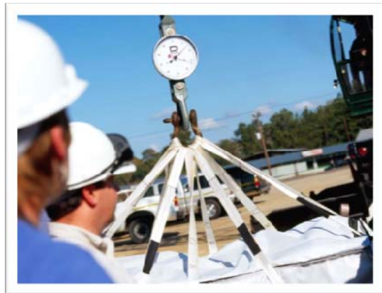
LiftPac bag lift test
