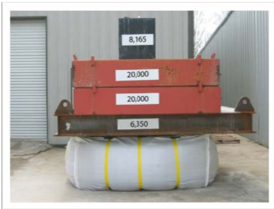
LiftPac bag stack test with 54,515 kg of weight
