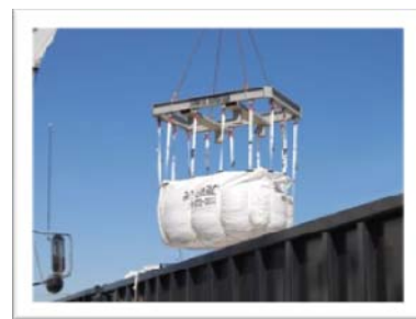
LiftPac bag loaded into rail wagon
