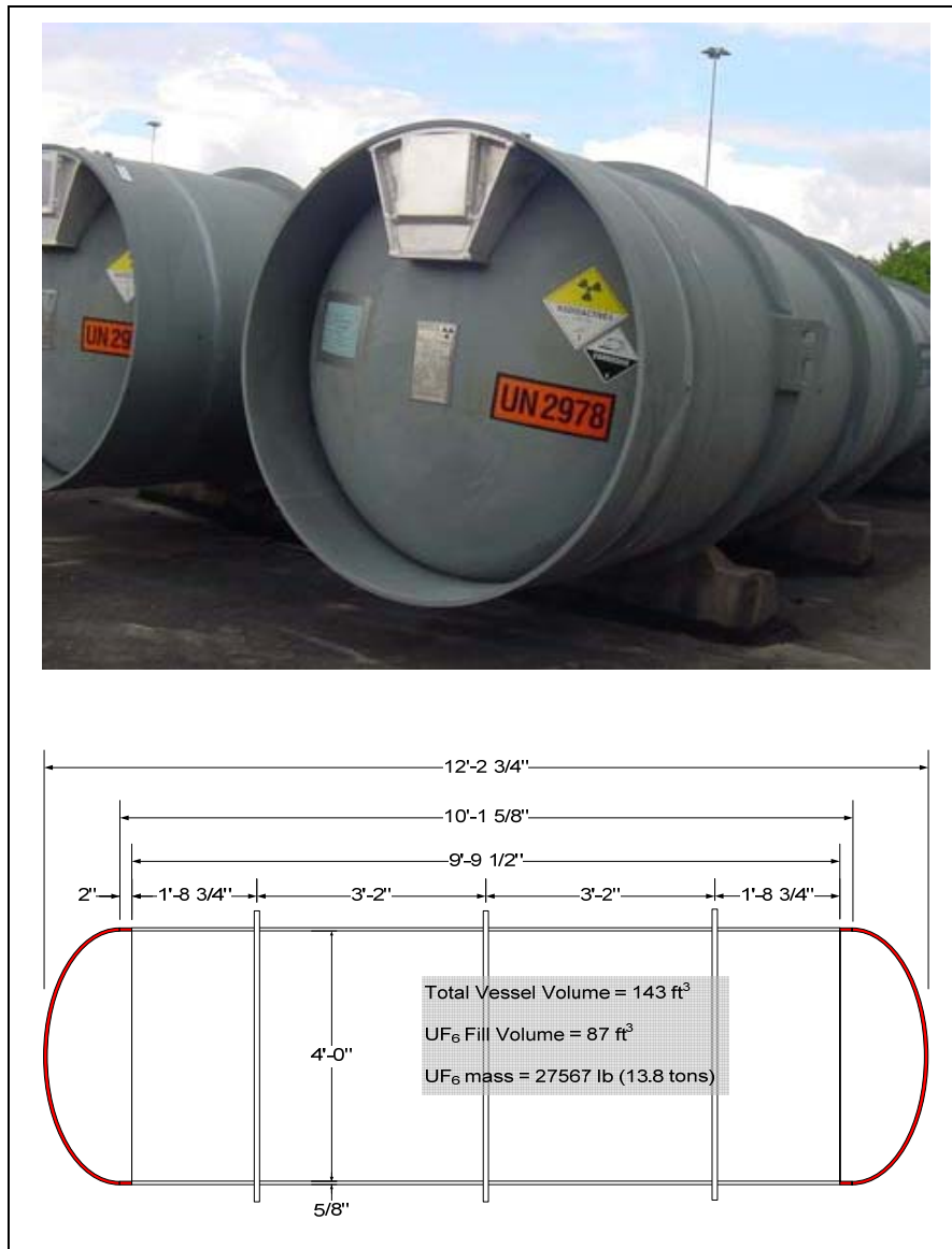
Figure 1. The 48Y UF 6 container
