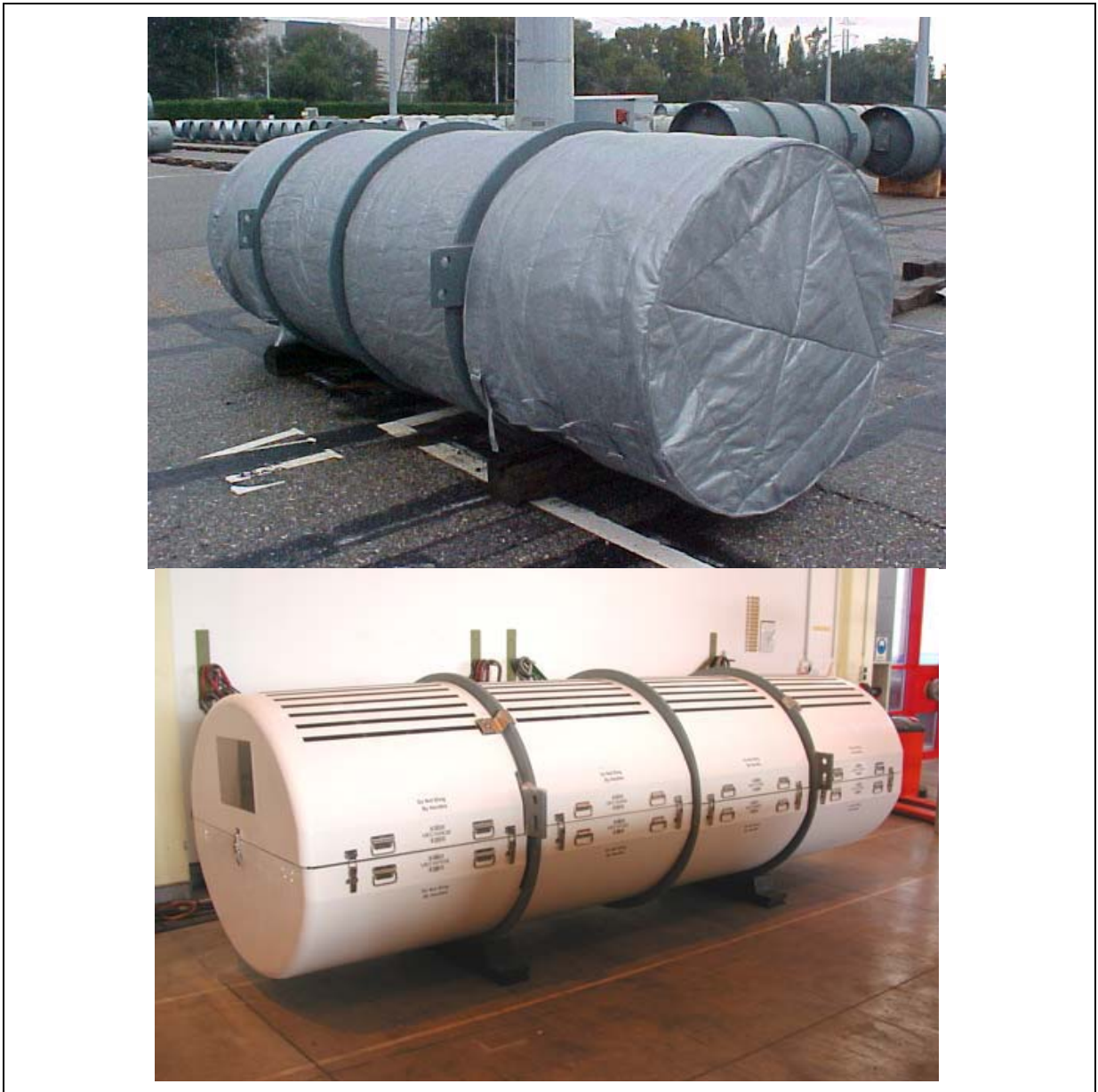
Figure 2. 48Y UF 6 container with the BTP (top) and the CTP (bottom)
