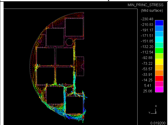
Figure 7 Stress flow in the second highest disc in the 0° hoop orientation in the 9m side drop
