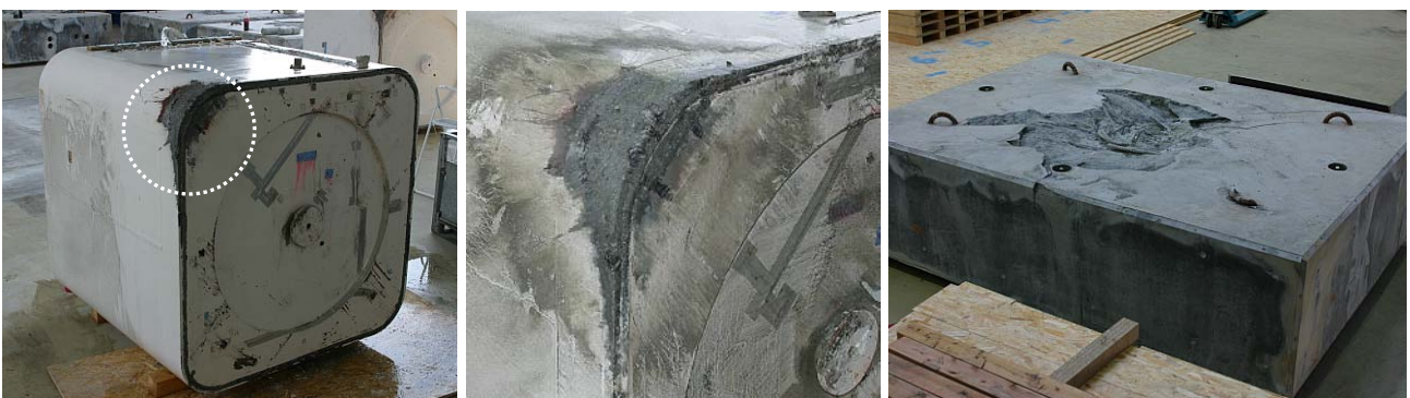
Figure 5. Specimen (left) and impact target (right) after drop test. Detail impacted corner edge (middle).
