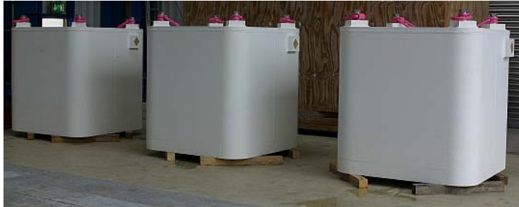
Figure.1. Specimen of the ‘Yoyushindo-Disposal’ waste container ready assembled for testing with different content masses.
