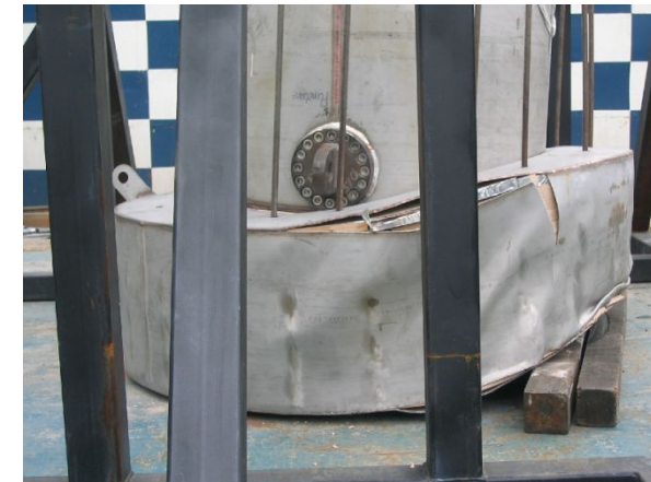
[Deformation in the impact limiter]
