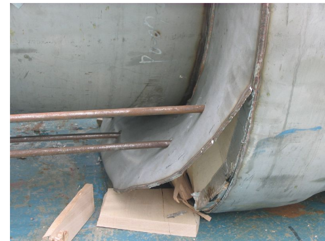
[Weld failure in the impact limiter]
