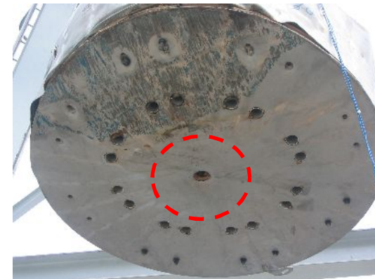
[Punctured shape at the impact limiter]
