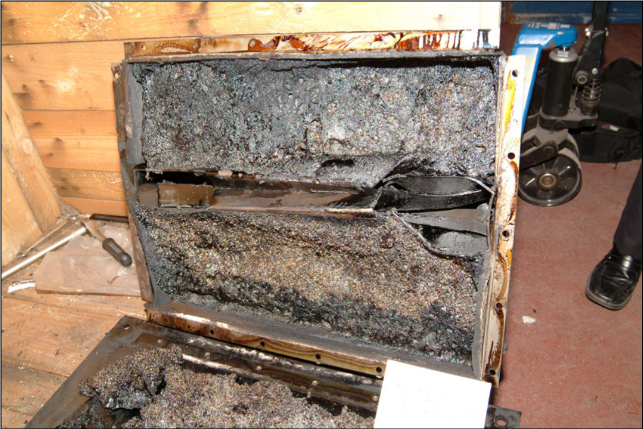
Figure 2. Effect on the Foam Following a Fire on the Other Side of the Test Box
