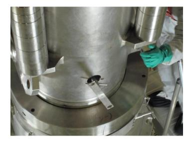
After docking of the transfer cask, the fuel pin was lowered in the R72 packaging, using the winch, and with the help of a camera to verify the correct insertion before undocking the transfer cask
