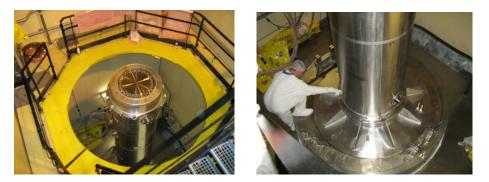
• cold testing in Nogent (F), in order to demonstrate the loading of the R 72 by placing the packaging docked under the pool.
