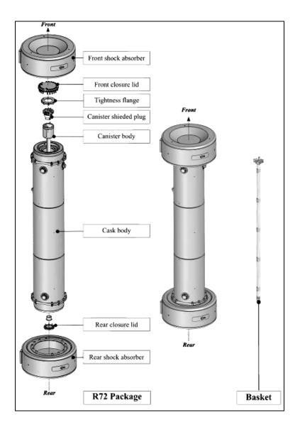
All included, it's a 21.5 tons cylindrical package of around 6.3 meter length, a diameter of 1.7m and 2 shock absorbers of 1 ton each. The package inner cavity is a  $5.3m \times 0.14m$  cylinder; it allows up to 10 fuel rods and tolerates a weight up to 650 kg.
