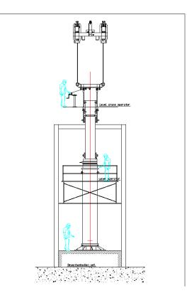
A footplate has been placed on the floor plate of the decontamination cell in the reactor building. This was done very carefully, as the total height of the combination R72 + transfer cask is about 10 meters high. Furthermore, the verticality was an important aspect, as the fuel pin had to be lowered in the basket of the R72 with very little gap.
