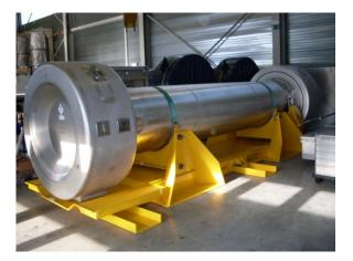
In order to be fully compatible with all labs where the fuel pins are loaded or unloaded, two different types of canister is existing; both canisters differ by the way of handling (one can be handled by existing fuel handling devices) and by their diameter of the head (the smallest one can be pushed through an opening of 250 mm)
