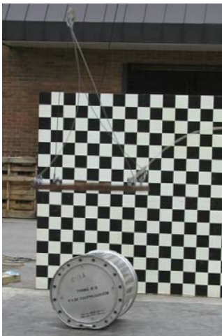
Figure 9. The crush plate just before impact with MD-2 TU-3.
