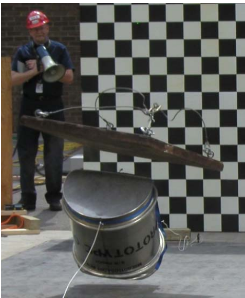
Figure 3. DPP-2 TU-2 recoils off of the drop pad in response to initial impact of crush plate.
