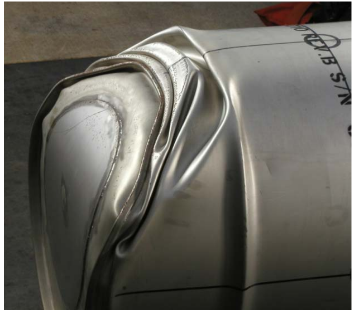
Figure 2. Crush test damage to ES-2100 TU-3.
