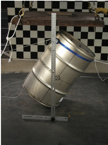
Figure 1. The CG of the crush plate is aligned with the CG of ES-2100 TU-3 before crush testing.
