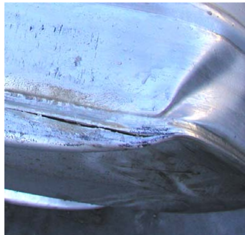
Figure 10. Split drum weld seam on MD-2 TU-1 after crush test.
