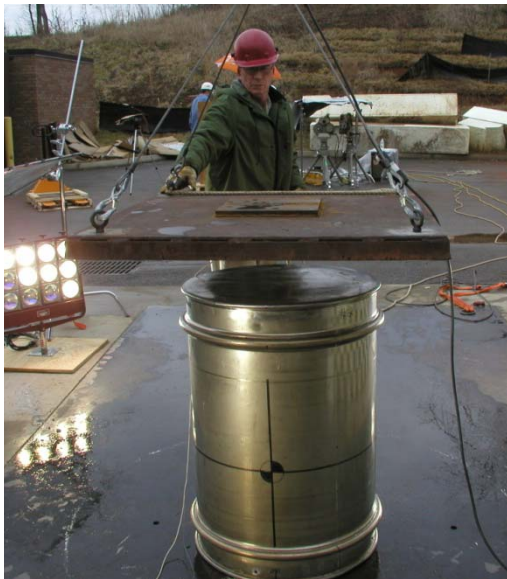
Figure 5. The crush plate is centered over MD-1 TU-4 before crush testing.
