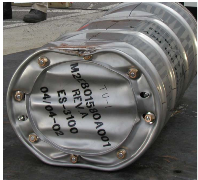
Figure 8. Cumulative 9 m drop and crush test damage to ES-3100 TU-1.
