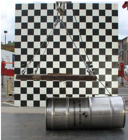
Figure 7. The crush plate is centered over the CV flange of ES-3100 TU-1.
