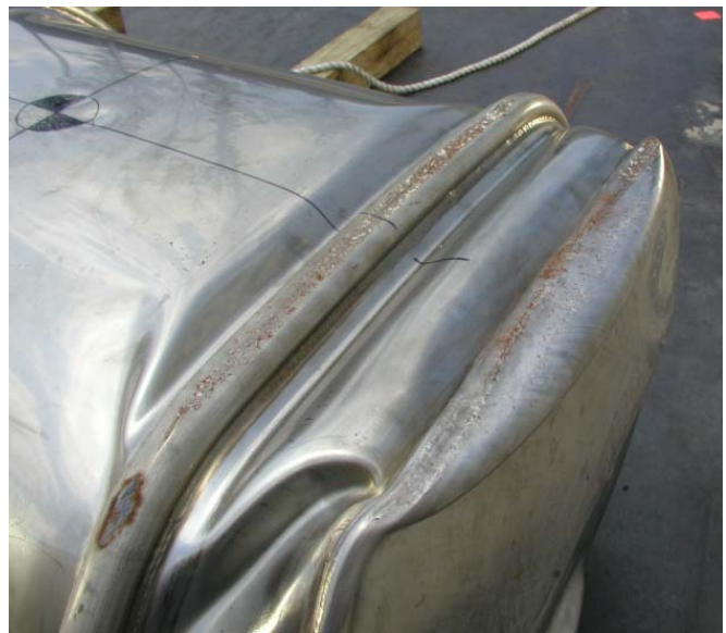
Figure 4. Crush test damage to DPP-2 TU-6.
