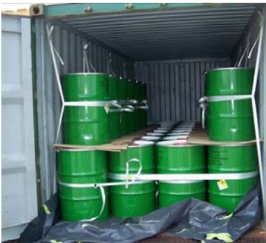
Figure 1: Stowage with lashings, 8 stacked drums, open head drums with a center hole in the lid
