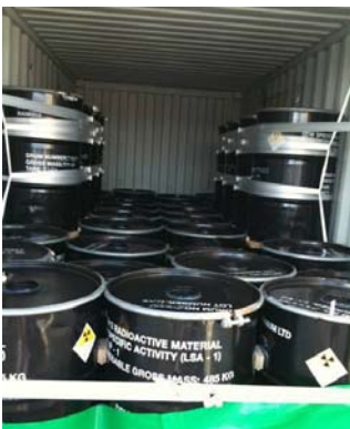
Figure 3: 8 stacked drums, open head drums with a center hole in the lid, drums supported by spacers of different thicknesses
