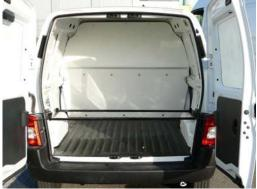
Lead shielding in vehicle plus physical restraints across the rear wheel arches.
