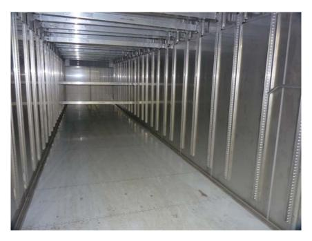
Lead shielded articulated lorry trailer with adjustable load bars.
