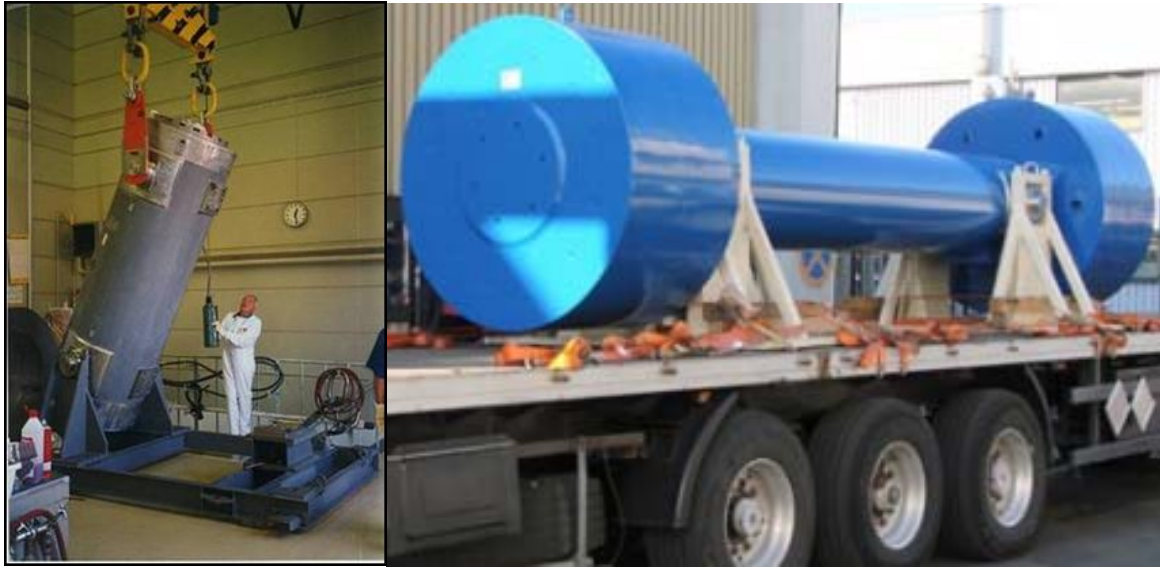
Figure 3. Tilting and trailer fixation of a cask
