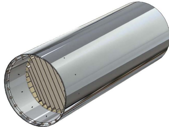
Rad Waste Container (RWC)
