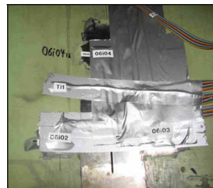
Figure 3. Notch with strain gauges
