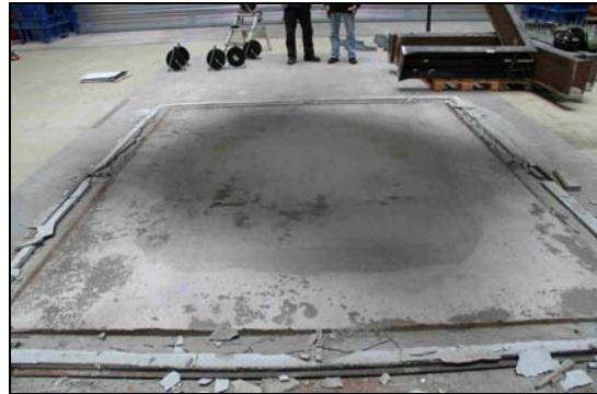
Figure 6. Mortar layer after drop test with optimized target construction
