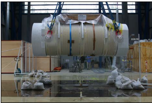
Figure 1. Cask before puncture drop test
