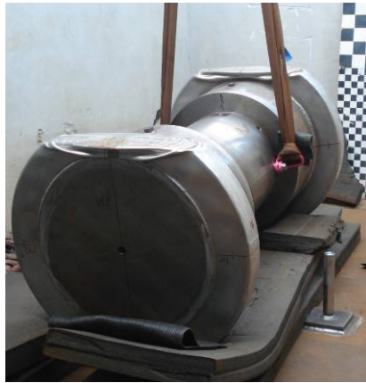
Figure 3. Picture of scale model of cask after lateral drop test
