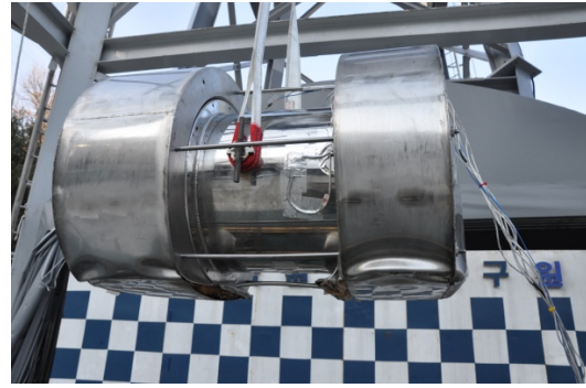
Fig. 3. Deformed shape of shock absorber.
