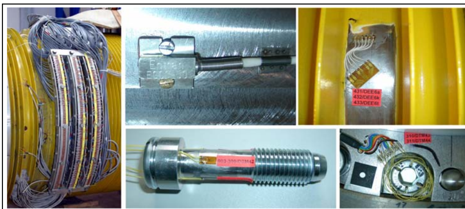
Figure 3. Central soldering terminal (left), accelerometer (top centre), strain gauge on the cask body (top right), strain gauge instrumented lid bolt (bottom centre and right)
