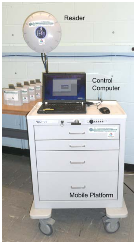
Figure 2. A stand-alone RFID temperature-monitoring system on a mobile platform (left) and an RFID tag mounted on a 9977 (or 9978) package (right).
