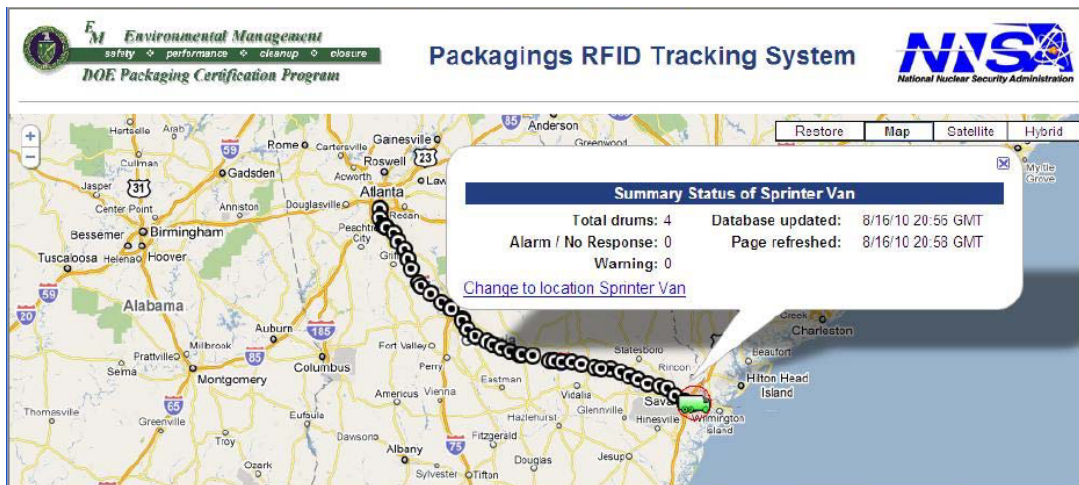
Figure 8. Screenshot of the ARG-US TransPort web page taken from a remote laptop during the road test of Sprinter van from Atlanta, GA to Savannah, GA, August 16, 2010.
