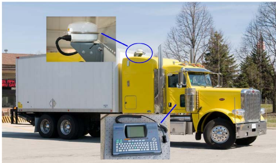
Figure 2. The "Big Bird" truck with the OmniTRACS satellite communication unit.
