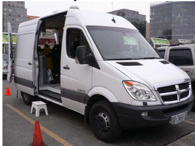
Figure 7. Sprinter Van used as a mobile platform for Transportation Security Technologies Testbed (The ARG-US TransPort control computer, RFID reader and MK-II tags are in the van; the OmniTRACS satellite transponder is mounted on the roof and the tablet is in the van.)
