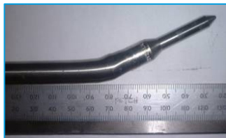
Buckling tests of fresh LWR fuel pin samples (tests 1 to 3)
