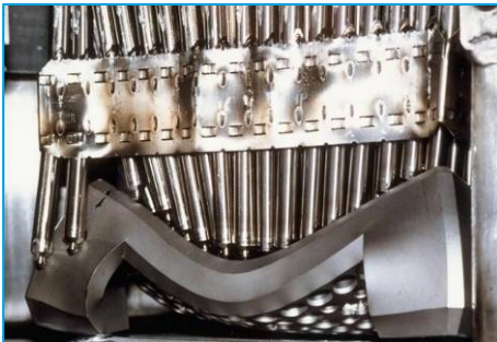
PWR 17x17 fresh fuel assembly loaded in the FS 69 cask
