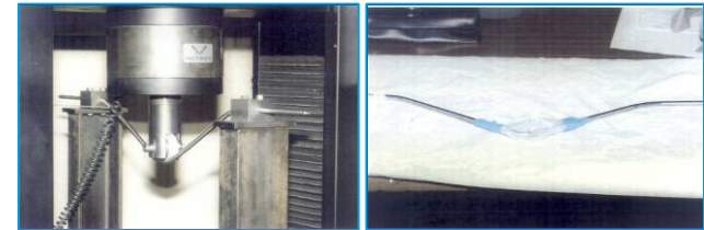
1987 bending test on PWR fresh fuel pins
