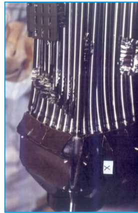
BWR 8x8 fresh fuel assembly loaded in the FS 74 cask
