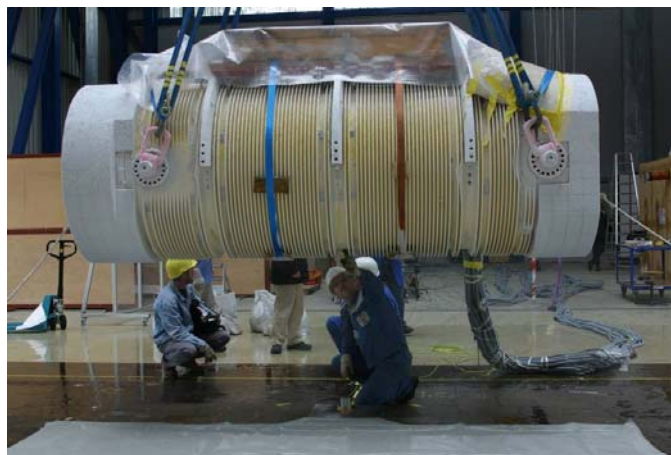
Fig. 1. Preparation of 1m puncture bar drop test at -40^{\circ}\text{C} (check of test parameters)
