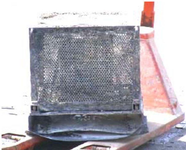
Package with external protective hull after fire
