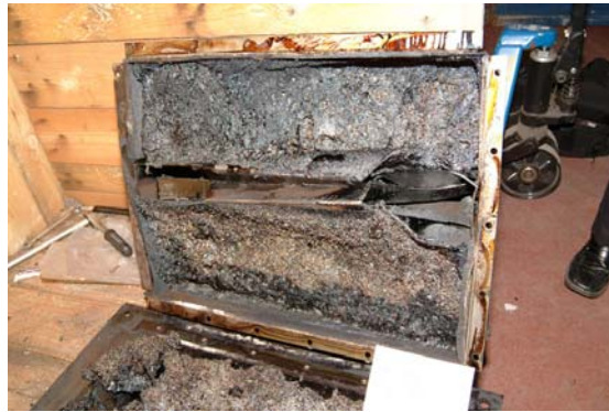
Figure 10. Panel Opened Following Impacts & Thermal Test to Show Burnt Foam
