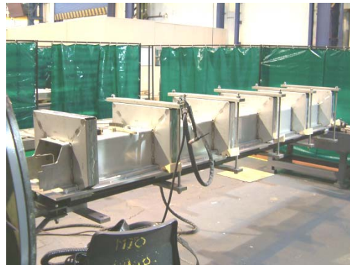
Figure 4. Body Under Construction, Showing Internal Stiffeners
