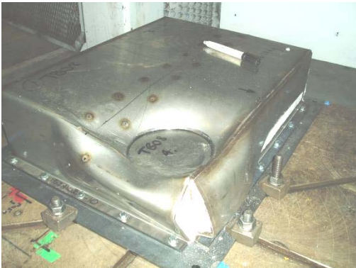
Figure 9. Specimen Panel, Following One Punch Impact
