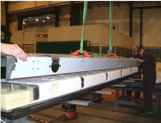
Figure 5. Lid in Build, Showing Foam and Blanket Materials
