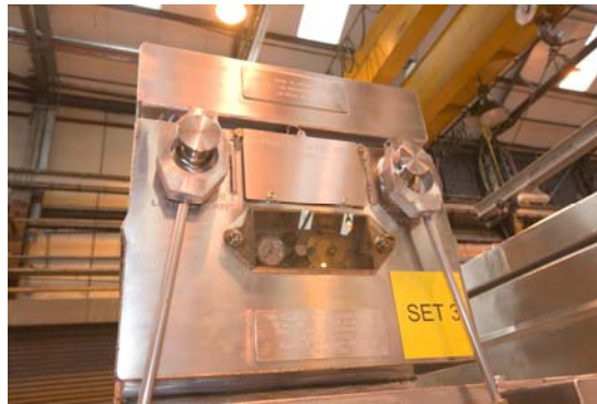
Figure 12 Pressure Fittings & Locating Features
