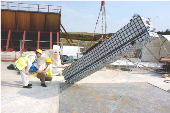
Figure 13. Setting-Up for Drop Test
