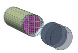
Overpack made of flat plates
