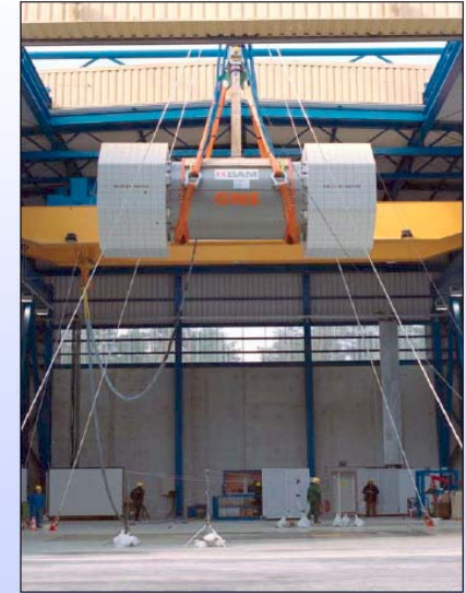
CONSTOR V/TC Full-Scale Drop Test 9m horizontal drop (Sept.2004)
