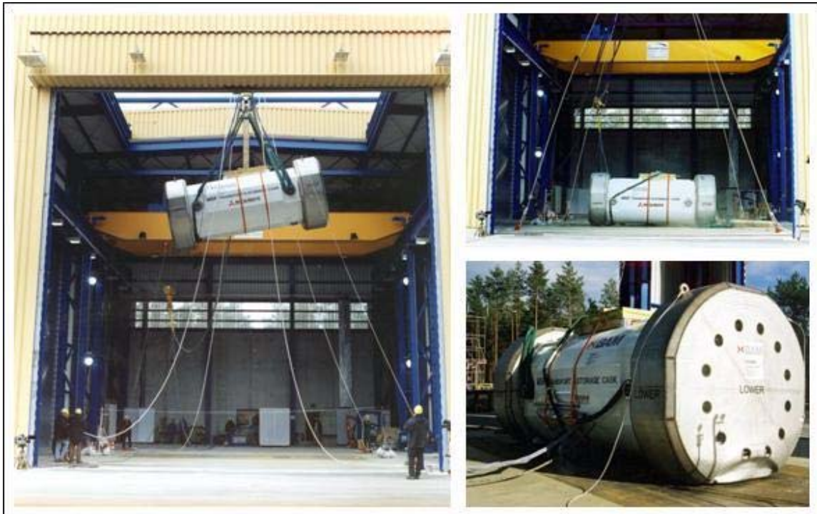
Figure 2.9 m slap-down Drop of MSF-69 BG full-scale Cask before (left) and after (right) Impact
