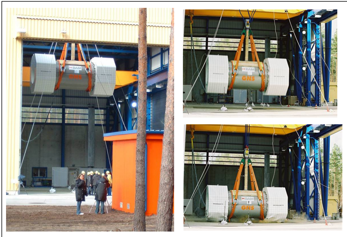
Figure 1.9 m Horizontal Drop of CONSTOR V/TC full-scale Cask
