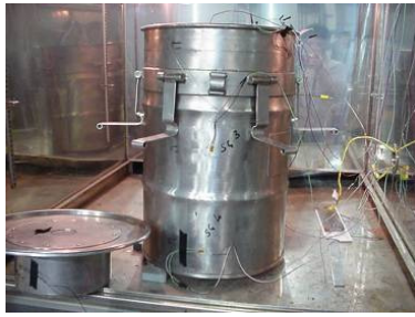
Figure 8- CF6 in the climatic cell and check on the material
