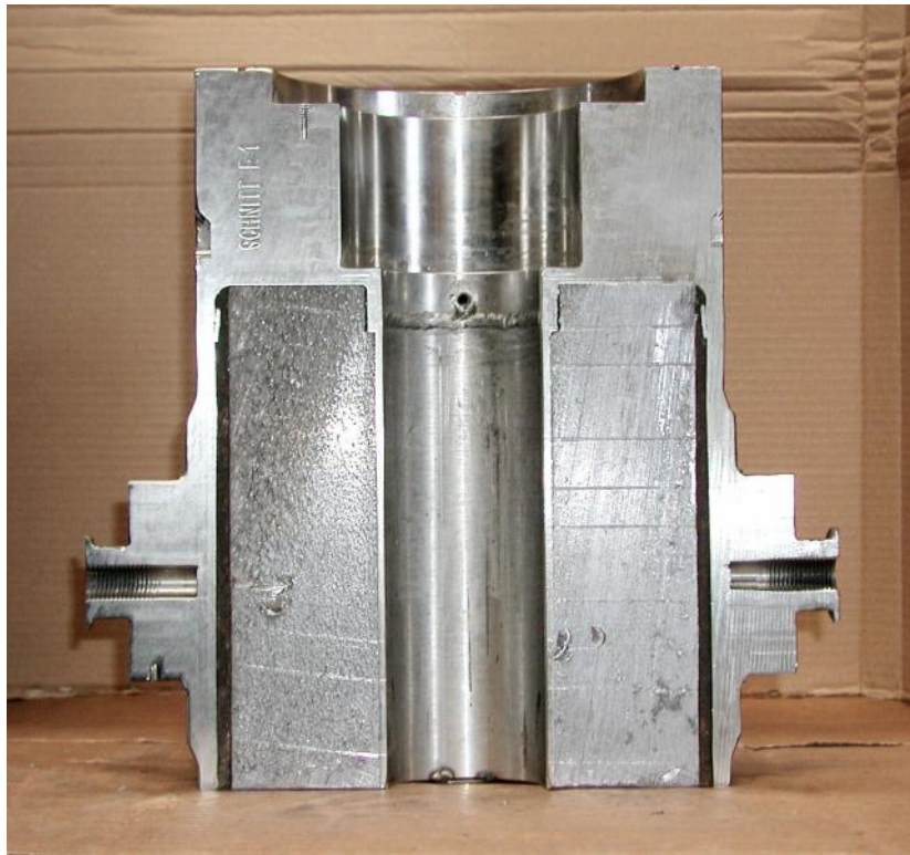
Figure 6. Cut Through the Bottom Part of the Drop Test Model – no Lead Slump
