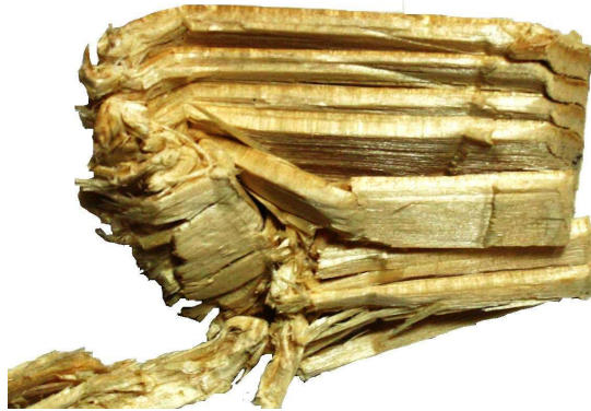
Figure 2. Buckled Layers of Fir Wood (BAM experiment, M. Neumann, 2007)
