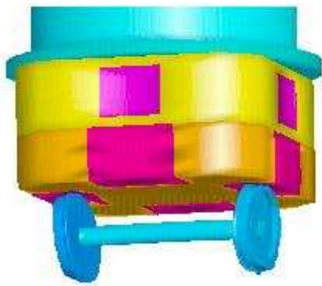
Figure 4. Impact of spent fuel package onto railcar axle
