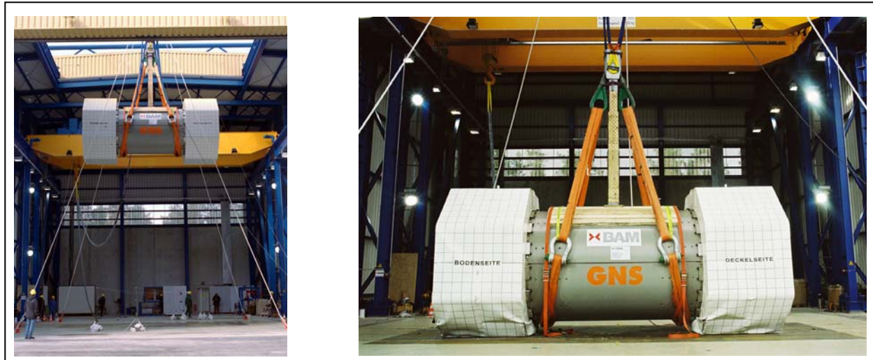
Figure 1. Nine Meter Drop Test of CONSTOR ® V/TC before (left) and after (right) Impact
