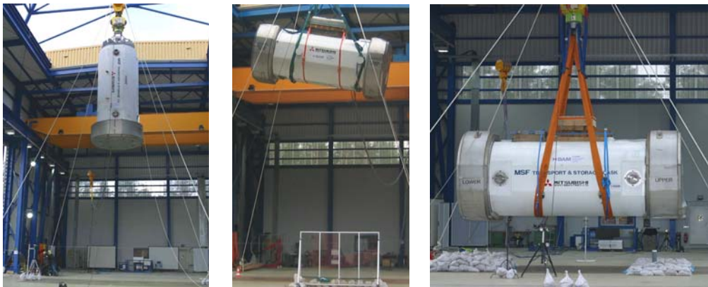
Figure 1. Drop Tests. Vertical, Oblique and Horizontal Cask Orientation.
