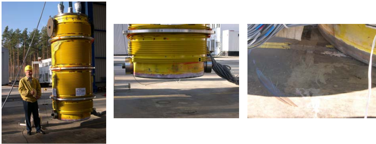
Figure 1. 0.3 m vertical drop test at BAM with CASTOR® HAW/TB2 onto BAM's 2,600 Mg IAEA target
