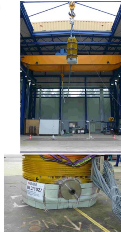
Figure 2. Test results of 0.3 m drop without impact limiter compared to those of 9.0 m drop with impact limiter
