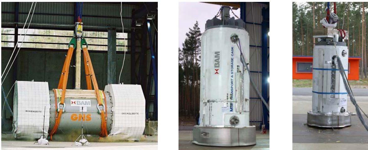
Figure 1. Test Containers TC1, TC2, TC3 (from left) just after Drop Test.
