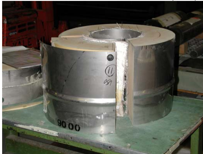
Figure 1. A 9977 package was sectioned to obtain in-situ specimens for material property tests.
