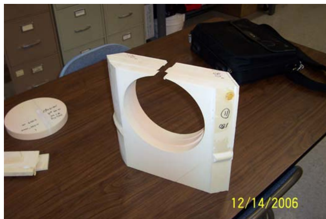
Figure 2. Thermal conductivity specimens were taken from the section of the side wall shown in Figure 1.
