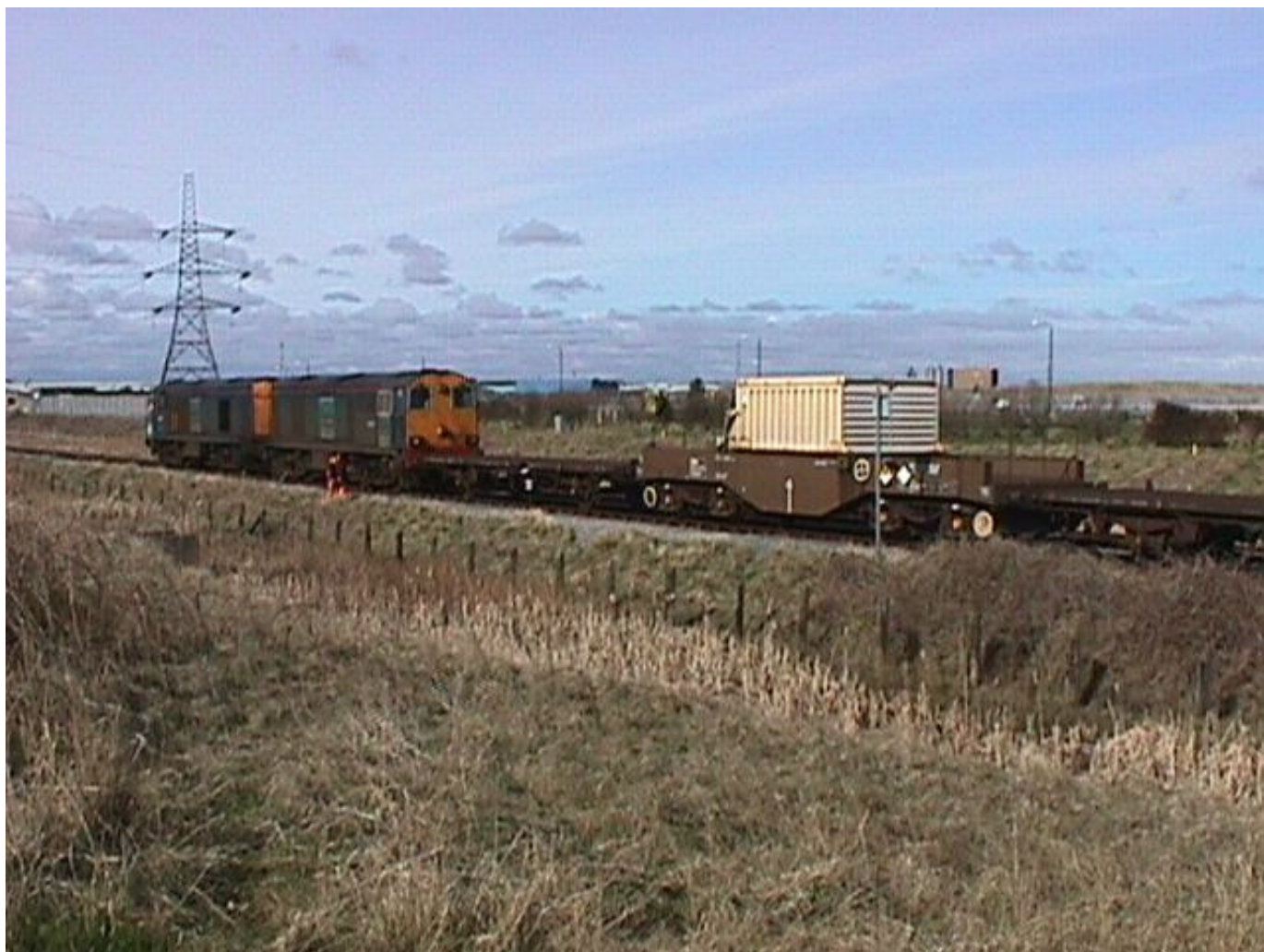
Figure 1: Train transporting an A2 fuel flask under covered rail flatrol
