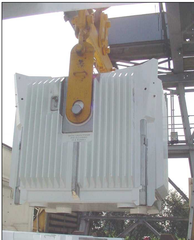
Figure 2: An AGR Mk A2 Irradiated Fuel Flask being handled at a railhead
