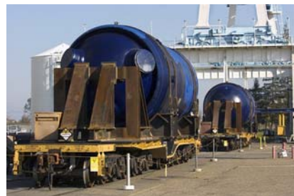
Figure 6. PBS Coating on Steam Generator
