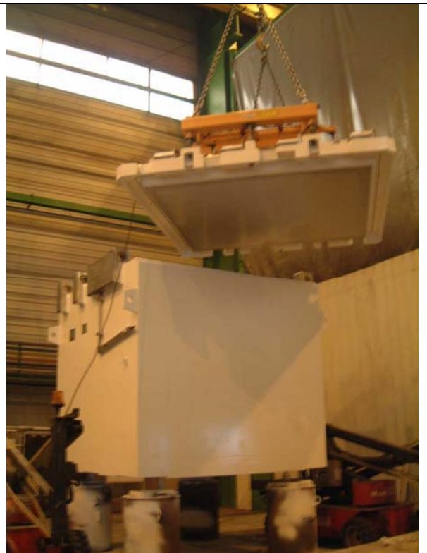
Picture n°6 = lid final fitting tests
