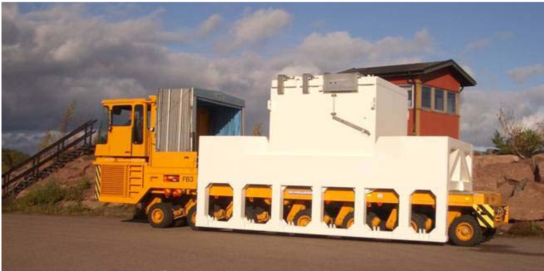
Picture n°2 = ATB8K on its frame on the terminal vehicle
