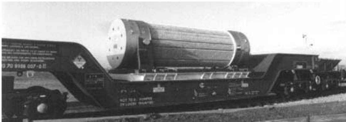
Figure 1 - BNFL Swan-neck Rail Vehicle with Spent Fuel Package
