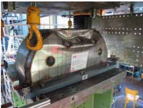
Figure 5. Shock Absorber Compression Test Results
