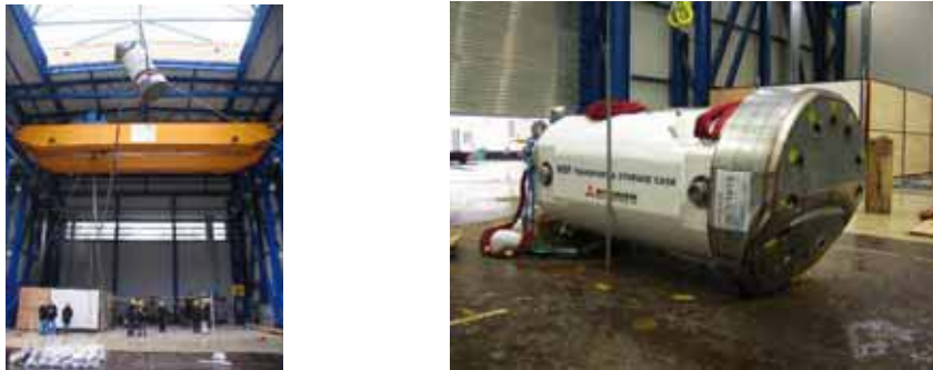
Figure 3. Oblique (Corner) Drop Test with 1/2.5 Scale Drop Test Model
