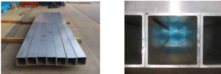
Figure 4. Basket Cells for Full-Scale Model after Series of Drop Tests
