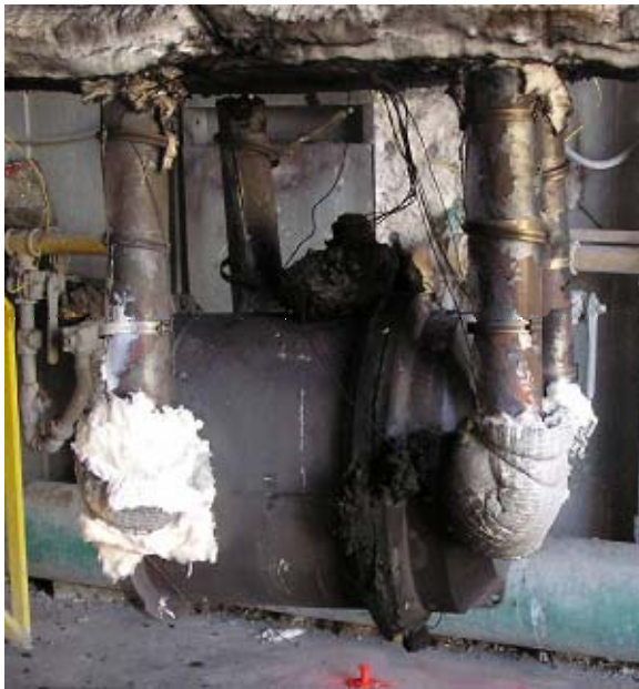
Figure 7 - Package Condition After HAC Thermal Test
