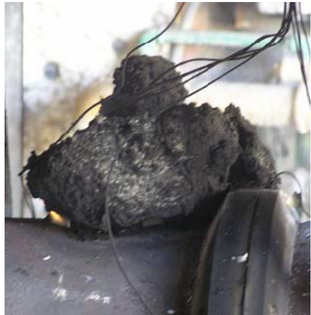
Figure 7 - Package Condition After HAC Thermal Test
