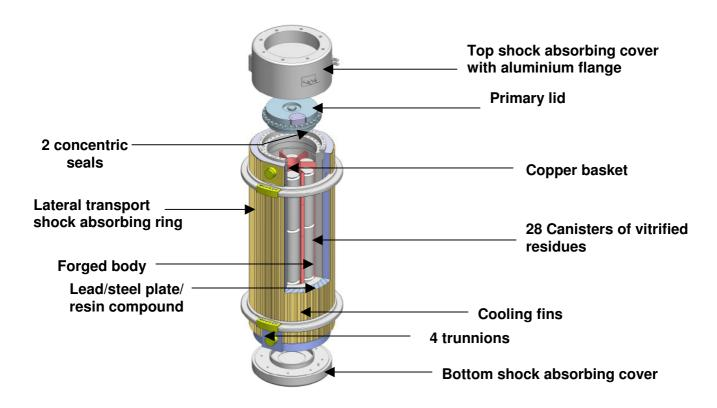
The transport and storage cask TN85 is intended for the transport of high level waste from the French reprocessing plant to a German interim storage facility and the following interim storage there.
