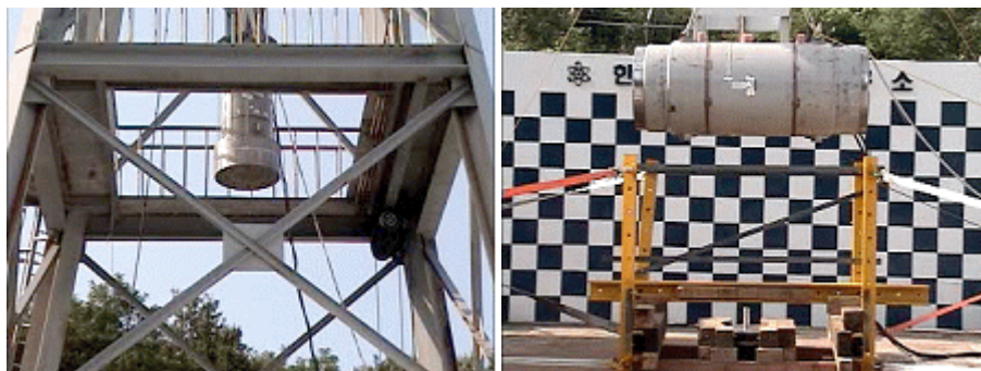
Figure 5. Drop(9 m) test and puncture test of spent nuclear fuel package
