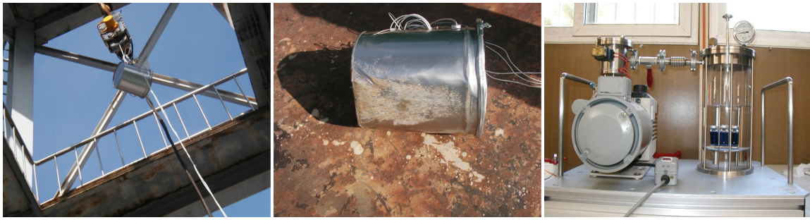
Figure 2. Drop test and vacuum bubble test for radioisotope package
