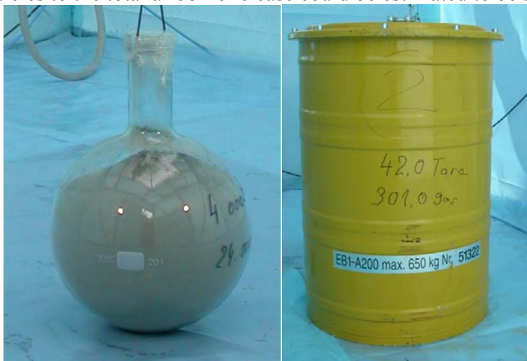
Figure 1. Different specimens used in the drop experiments. Left: powder in a thin 20 l glass flask (unclad); right: 220 l type drum, IP-2/Type A (clad)
