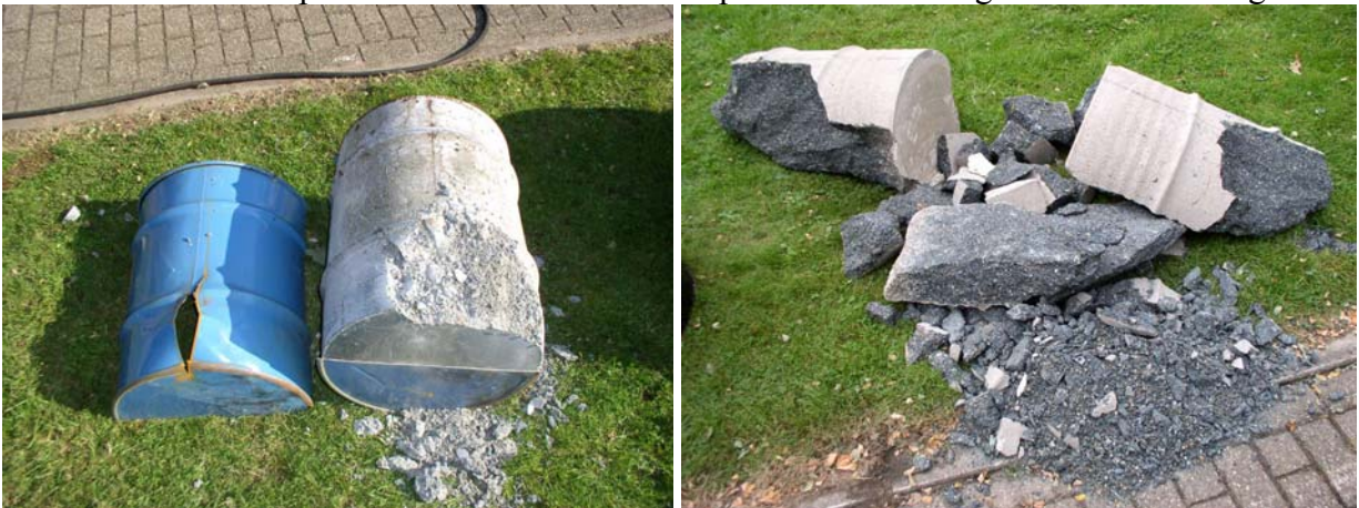
Figure 2. Damage and collected debris of the clad and unclad 220 l-drum after being dropped from a height of 27 m
