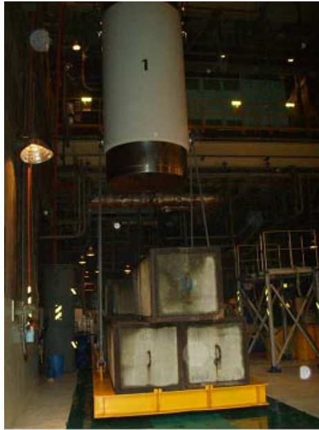
Figure 4. Load Inspection of the Cask.
