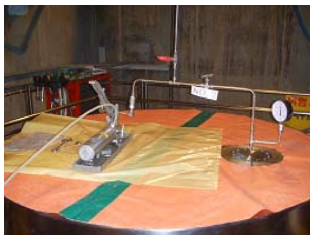
Figure 5. Pressure Inspection of the Cask.
