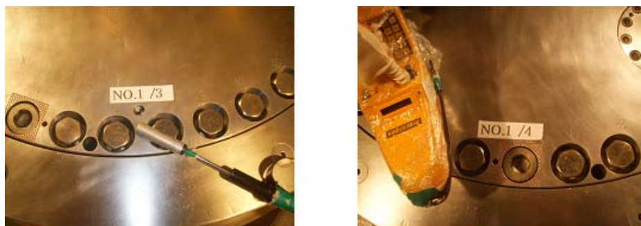
Figure 7. Measurements of the Gamma and Neutron.
