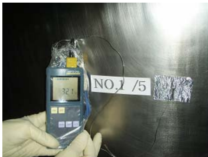
Figure 8. Measurement of the Temperature.
