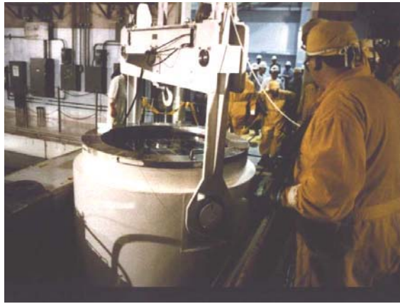
Figure 1 Loading TN 68 Dual Purpose Cask
