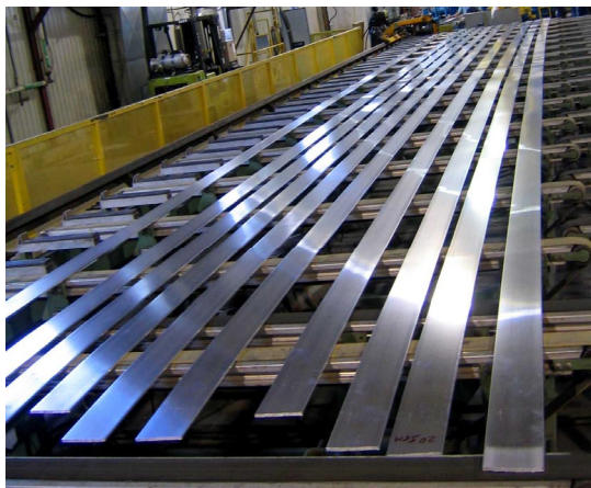
Figure 2. Extruded Bars of Boron MMC
