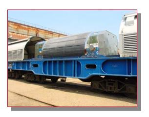
The TN 12 family flasks are characterised by thick forged steel body (about 300 mm).
