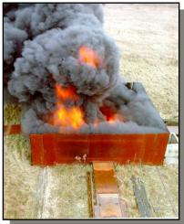
Following the test, the leaktightness of the FS 47 packaging was measured. It was still better than  $10^{-8} \text{ Pa.m}^3.\text{s}^{-1}$ . In other words, the fire test did not alter the leaktightness of the package.
