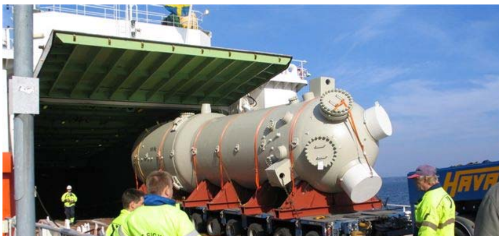
Figure 4. Unloading of a steam generator from M/S Sigyn.
