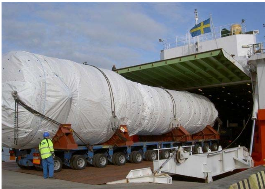
Figure 3. Loading of a steam generator on the INF 3 ship M/S Sigyn
