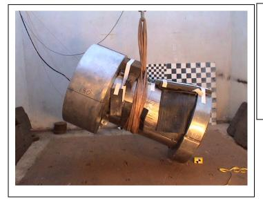
The development of the IR 800 included three halfscale test campaigns performed at AREVA TN International drop test station in the south of France.
