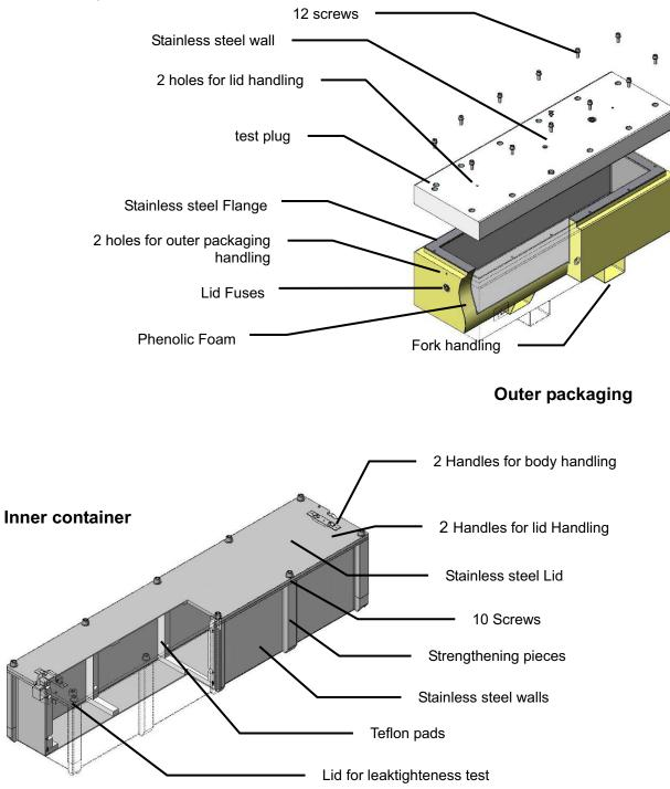
The FS 110 packaging with a total gross weight of 840 Kg and the main dimensions of 1919 x 733 x 630 mm consists of an outer packaging and an inner container. Both inner container and outer packaging are waterproof in order to avoid taking into account flood water in the criticality calculation.
