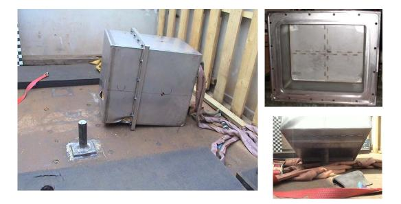
Drop test with leaktightness tests have been successfully performed at the TN International Laudun facility during 2006 fall. 9 drops with 5 puncture tests were necessary. No major deformations have been induced by the puncture tests or 9 meter drop tests. Strengthening cross, anti-punching aluminium plate and flange have perfectly resisted to all the stresses.
